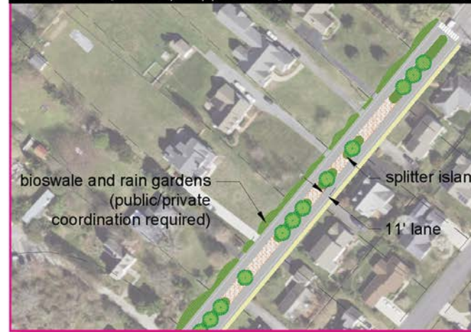
Traffic Calming Concept Approaching 4th Street (w/infiltration)
