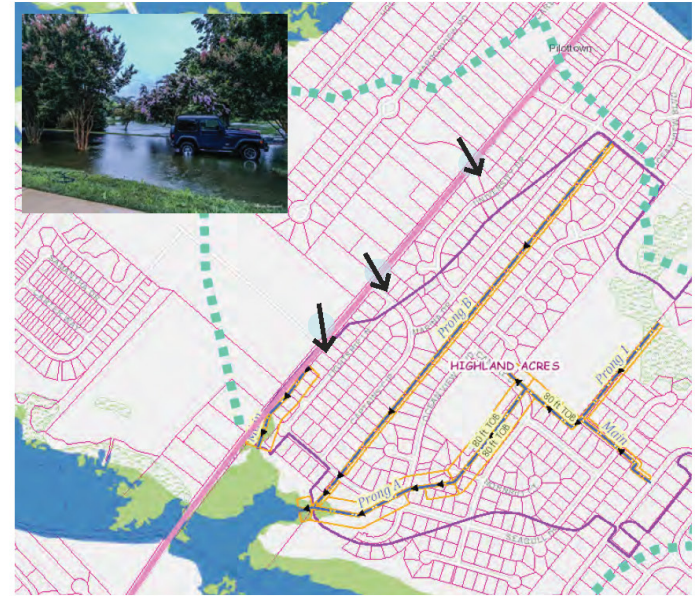
Figure 80 Catchment Area for the WB side of New Road feeds to culverts (blue circles)- NTS
