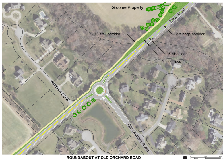
Figure 72 Sections illustrating splitter at Arkansas Court (top) and Roundabout at Old Orchard (bottom) - Roundabout dimension shown is minimum, actual dimension TBD
