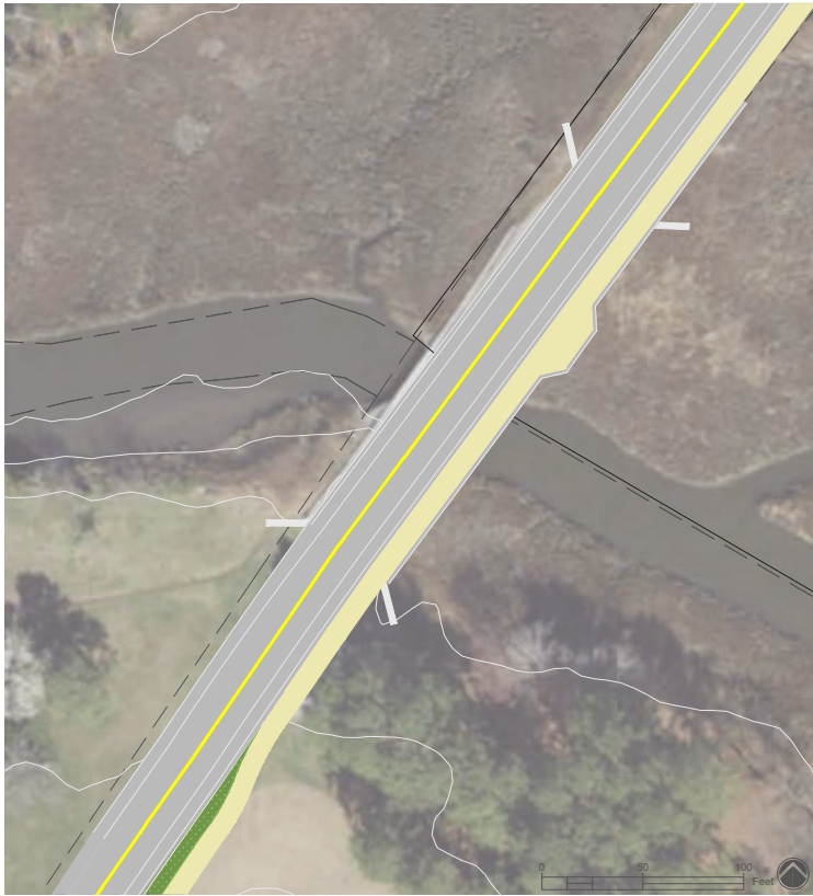
Figure 85 Illustrative concept showing a combined structure used to accommodate both the vehicular travel lanes and the shared use pathway with an overlook to Canary Creek
