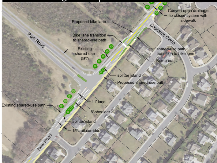
Figure 87 Concept plan or recommended modifications to the Park Road intersection with splitter island examples
